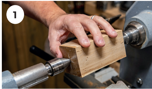
1. Mount your blank between centres, this blank measures 125mm x 50mm.
