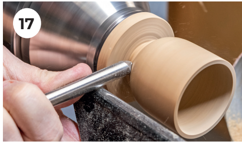
17. Now finish the shaping around to the parting tool cut, this is best done with a small bowl gouge.
