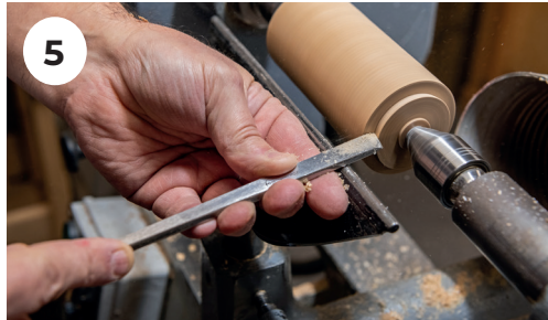
5. Cut the tenon into a slight dovetail.
