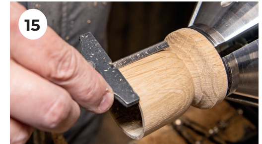
15. Check the depth before parting off to ensure you don't cut through the bottom.
