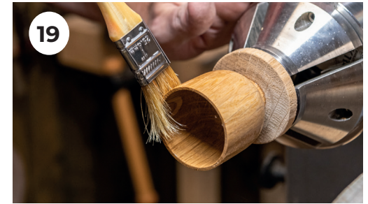
19. Coat the box in sanding sealer, wipe dry and lightly sand back.
