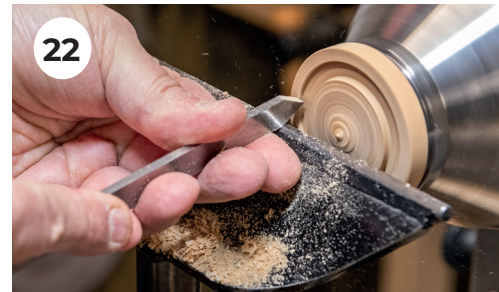
22. To finish the base, make a jam chuck from a piece of scrap wood.
