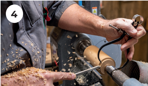
4. Cut a tenon to this size on the tailstock end of the blank.
