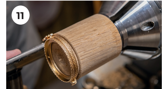
11. Test fit the hinge to ensure a good snug joint.
