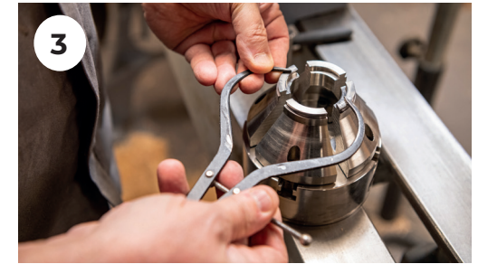
3. Using a set of O'Donnell jaws (610357), open to the optimal size (true circle) and measure the internal with callipers.
