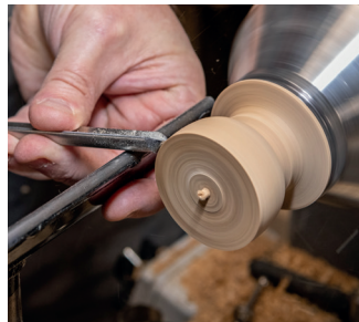
22. To finish the base, make a jam chuck from a piece of scrap wood.
