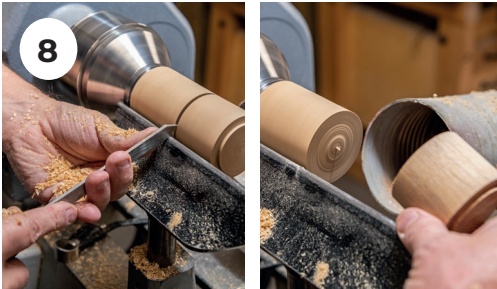
8. Using a parting tool, part off the lid section at 50mm.
