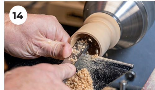
14. Finish off the shaping of the round bottom with a round nose scraper to blend in the curves.
