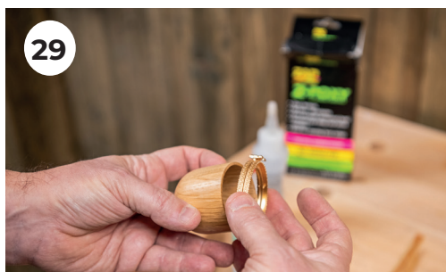
29. Using epoxy, glue the lid to both base and top.
