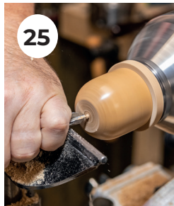
25. Using a bowl gouge tidy up the base, sand and polish.
