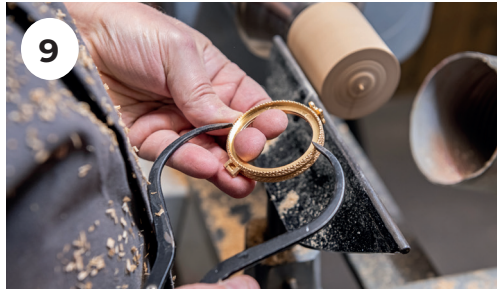
9. This will leave you the base section in the chuck and ready to start sizing for the lid. Using callipers measure the inside diameter of the hinge.
