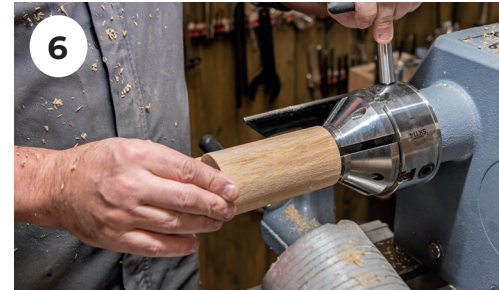
6. Remove from between centres, mount chuck onto the lathe and hold the blank in the chuck
