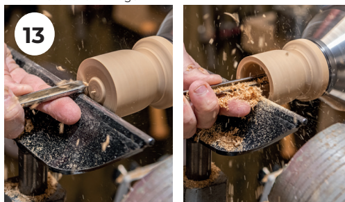
13. When happy with the external shape you can hollow the inside using a bowl gouge.
