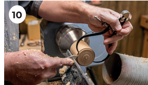
10. Now cut a tenon to suit the hinge measurement.
