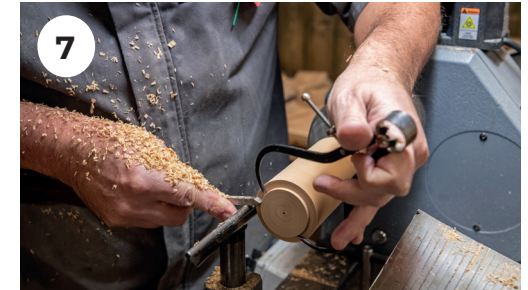
7. Cut another tenon on this newly exposed end, the same size as before and once again cut to a dovetail.
