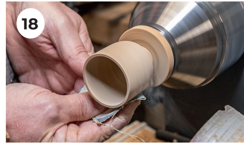
18. You are now ready to sand the inside and outside of the box making sure you do not over sand and make the box under-size for the hinge.
