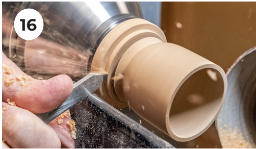
16. Knowing where the inside hollow stops you can make a small depth cut with a parting tool.
