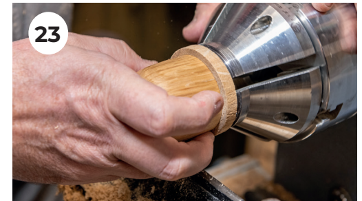
23. Cut in a recess to jam the box into.
