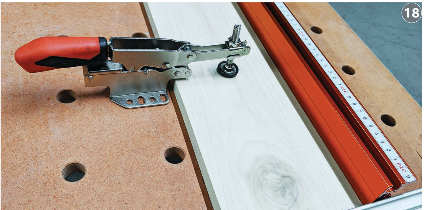
18. This UJK toggle clamp is a useful accessory for holding your workpiece securely.
