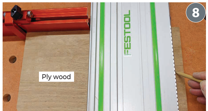
08. Find a straight edged piece of ply or planed timber, 4-500mm long and place it under your saw guide rail with the front edge protruding 50mm or so. Bring the flip over stop up to the rear edge to hold the ply or timber in place. Either run your saw to scribe a cut line, or draw a pencil mark against the sacrificial strip on the saw guide rail.
