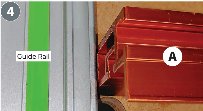
04. Fit your Guide Rail to your table, using dogs and Guide Rail Clips or Clamps. Slide the fence rail (A) up to the Guide Rail so that it touches firmly.
