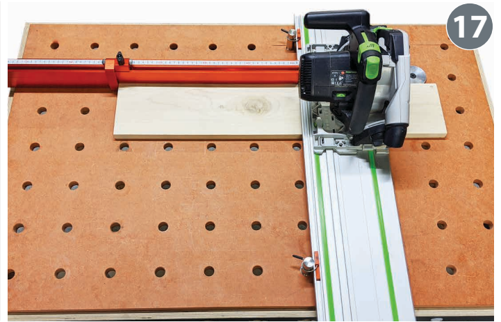
16-17. Refit your saw guide rail and you're ready to start cutting accurate lengths.
