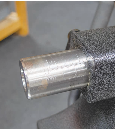
Tailstock barrel with integrated scale
