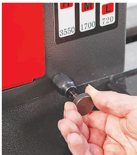
Pull out the pivot lock pin to rotate the headstock around with four preset angles, 60° - 90° - 120° and 180° degrees
