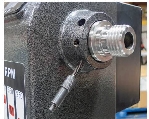
• Lower threaded hole for 36 point indexing
