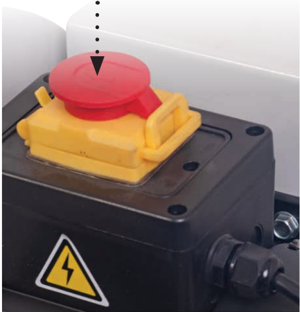
Emergency stop "SLAP" the shroud down to "STOP" the machine
