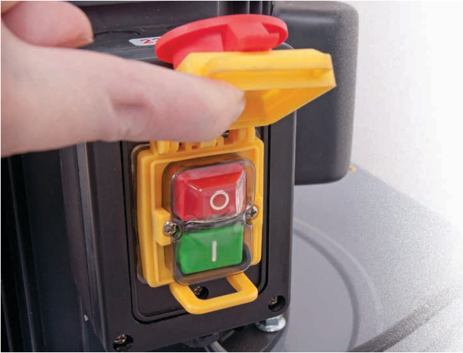
NVR switch assembly with (O) indicating (OFF) and (I) indicating (ON).
