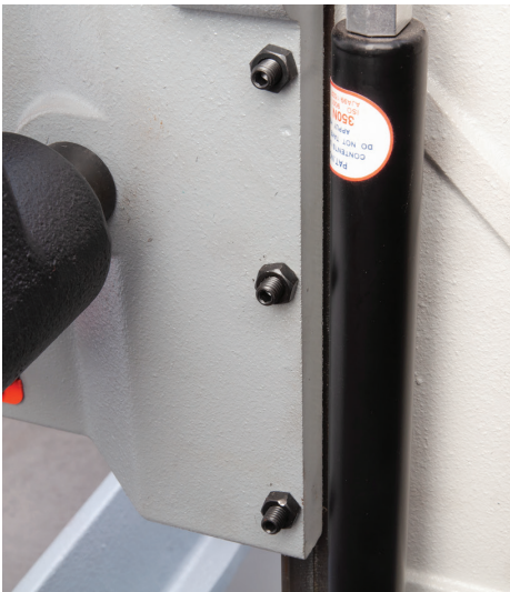
Gib strip adjusting grub screws and locking nuts
