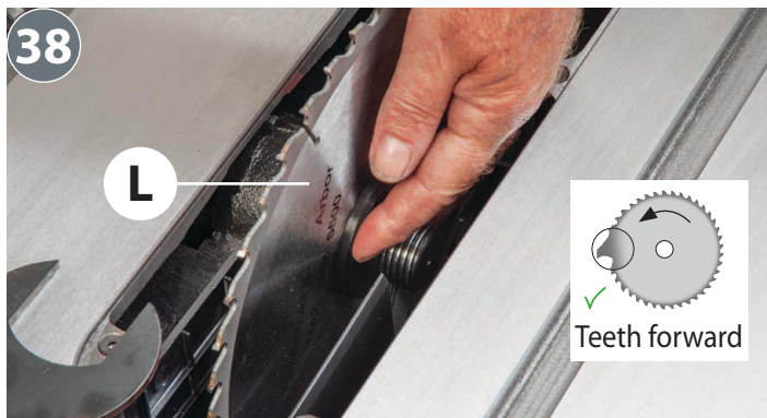
Slide on the blade (L) so its up against the rear flange
