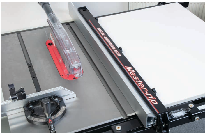
Rip-fence in the upright position for guiding timber through
