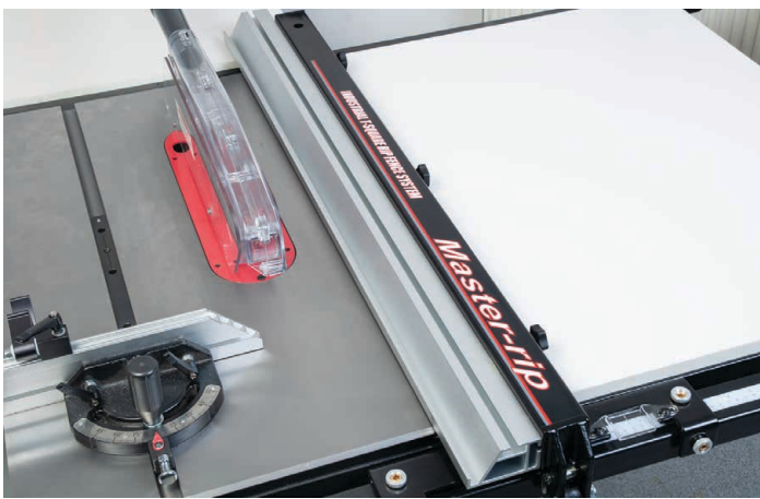
Rip-fence in the down position for guiding narrower timber through
