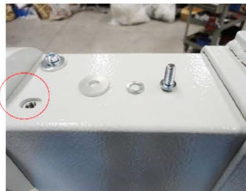
6 Insert the dust bracket into the fixed bracket then push it inside the fixed bracket
