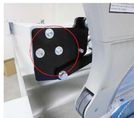
8. mount the saw blade guard to the support bracket , tighten the screws, lock washers and washers to steady it.
