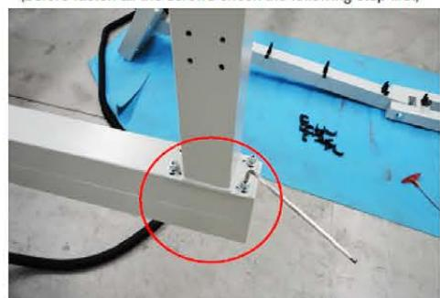
10. If the saw blade gaurd doesn't parallel with the blade, adjust the four screws from support frame.
