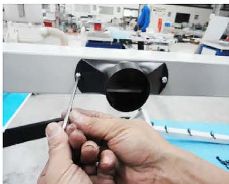
11. Install the dust hood to the support bracket, tighten the screws and lock washers (X2) to insert the dust hood into dust bracket.
