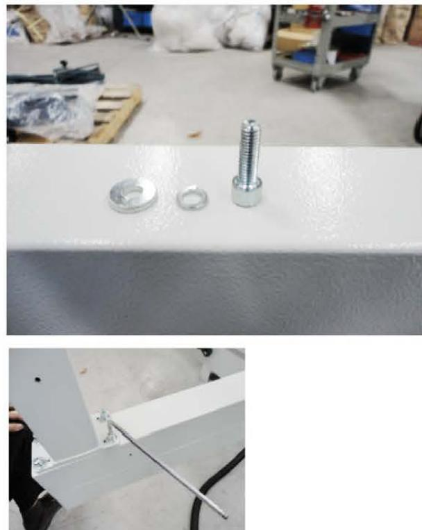
5 Put the fixed bracket on the support frame and aim at those four holes, then tighten the screws, lock spring washers and washers
