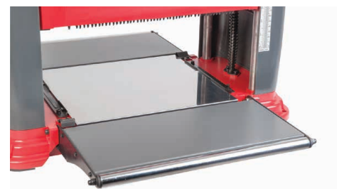
Width guides (E-F) keep the timber within the boundaries of the cutter block
