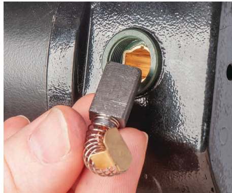
Remove the motor brush and check its condition
