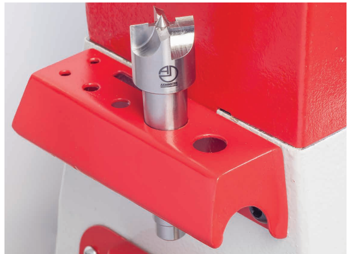
Tool holder/carrying handle on either end of lathe bed
