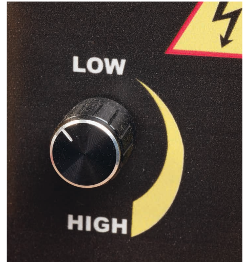
Variable speed control knob 250-3,550rpm
