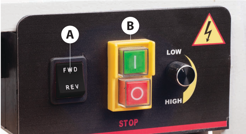
Forward/Reverse switch to change the spindle's direction (A) (DO NOT operate this switch while lathe is in motion) ON/OFF NVR switch (B)
