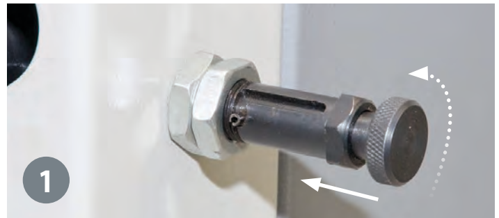
Preset stop bolt set at 90° degrees
