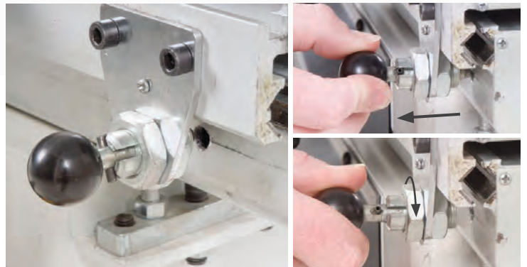
Sliding table locking knob Pull out the knob and twist
