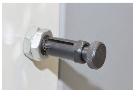
Spindle preset stop pin set at 90^{\circ} degrees
