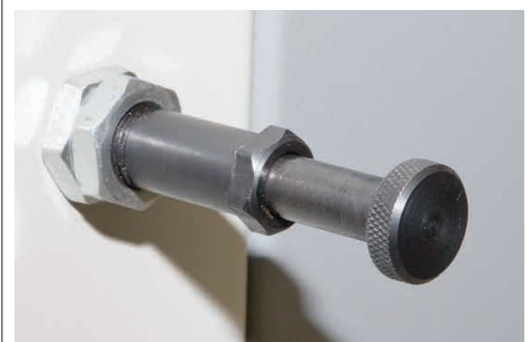
Spindle preset stop pin set at +05^{\circ} degrees
