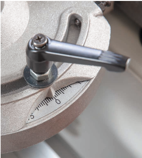
Fence mitre scale, pointer and clamping handle
