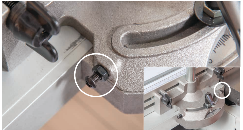
Fence mitre adjusting screw stops for -45^{\circ} to +45^{\circ}
