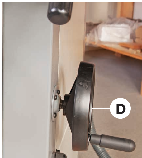
Rise and full control wheel (A), Control wheel locking lever (B), Blade tilt locking knob (C) and 45° Control wheel (D)
