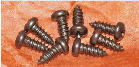
Eight small Phillips screws for mounting the capping plates above.
