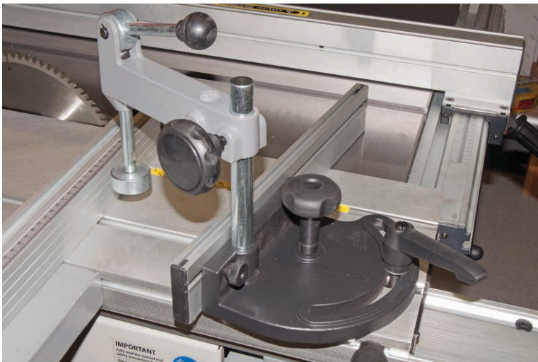
Sliding table mitre fence with over head clamp (A), Fence angle clamp (B), Over head clamp (C)
