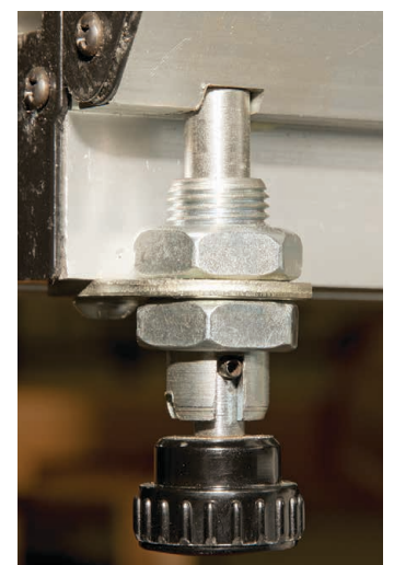
Sliding locking pin assembly Twist the knob to engage or disengage the locking pin
