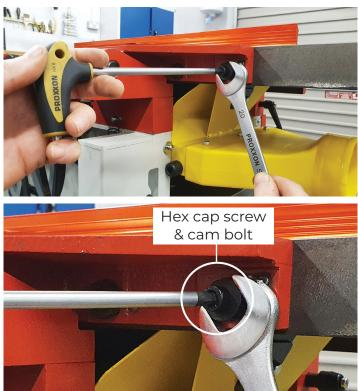
**4.** Adjustment will be also needed on the locking (front) side of the table to match the hinge side. With the table in its down position & lightly locked undo the 17mm nuts with a hex key in the grub screw.
