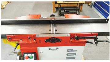
**8.** Refit front & rear panels then the fence bracket.
