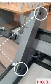
3. To align the fence to the blade/mitre fence slot the fence has been fitted with 2 grub screws that can be located here. FIG. 3
