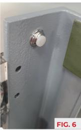
6. If the fence seems out of square to the table, then adjustment can be made by firstly unlocking the fence then winding the 2 nylon grub screws in or out. Adjust, relock then recheck for square, adjust again if needed. FIGS. 5 & 6
