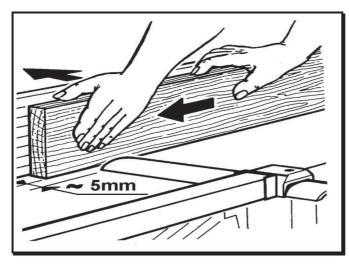
When planing narrow pieces set the cover of the cutterblock in such a position, so that the distance between the workpiece and cutterblock cover is max. 5 mm. Then switch on the machine and push and shift machined.workpiece against cutterblock (between the cutterblock cover and ruler).
