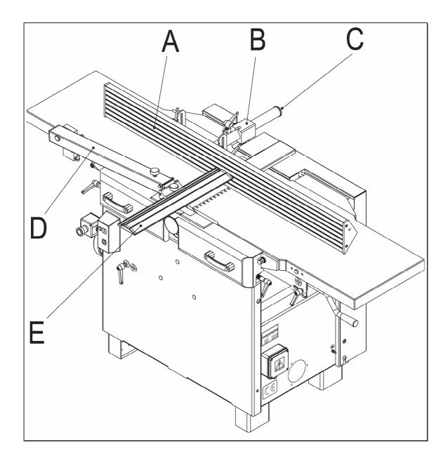
Into holder ( $\mathbf{B}$ ) insert tiltable fence ( $\mathbf{A}$ ), on the end of guide bar fix end stop washer ( $\mathbf{C}$ ). Adjust the fence according to the instruction (chapter 9.1.2)
