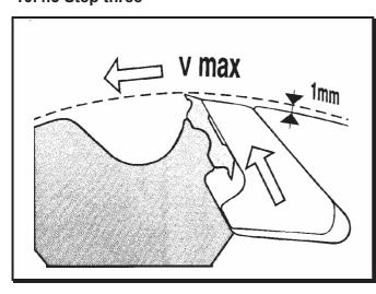
Eccentric power fixes the position of knives in cutterblock after starting the machine.
