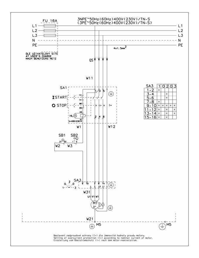
**Diagram 018-3-1** (3,7 kW, 3x400 (230) V, 50 (60) Hz, main switch, connection box, stop-button, brake release)
