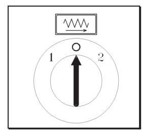
The thicknessing feeding drive of MSP 415 (SP 410) can be provided by a 2-rotation speed-electric motor.,
