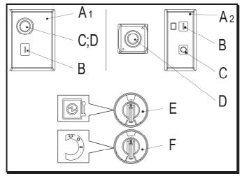
The machine gets connected or disconnected from the mains by pushing plug into or towing it off the mains socket, eventually by switching on/off the lockable main switch **E**. As long as machine is not connected with the mains-it cannot be started by operation switch **A**.
