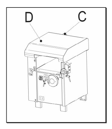
Exhausting nozzle (C) is fixed part of tiltable cutterblock cover (D).
