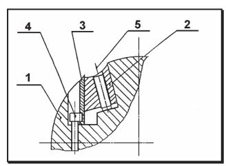
Swing away the planing tables before exchange of knives. Release three screws (5) in the pressing-off-wedge (2) by a hexagonal spanner nr. 4. Release the pressing off wedge (2) by hammer (through a piece of wood). Remove the knife (3) by unscrewing two hexagonal screws (4). Clean the wedge fitting surface and the new knife carefully. Insert the new knife by screwing two hexagonal screws (4) so as its maximal protrusion over cutterblock perimeter is 1 mm.
