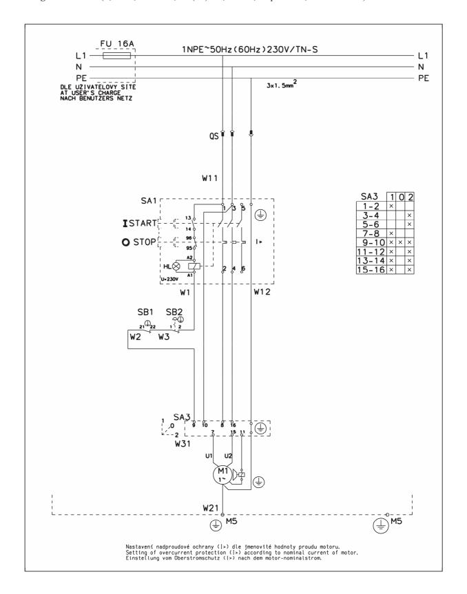
**Diagram 015-1-1** (2,2 kW, 1x230 V, 50 (60) Hz, socket, stop-button, reverse, brake release)
