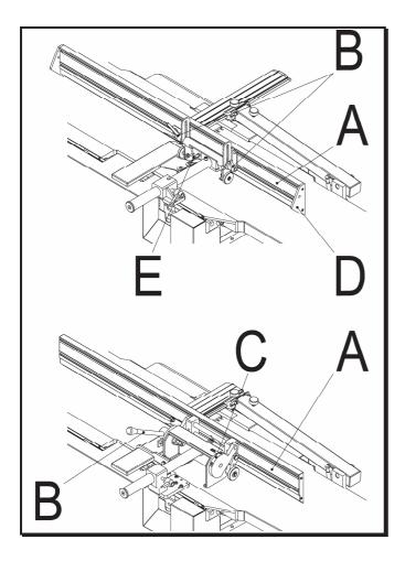
For tilting the surface planer fence (A) from  $90^{\circ}$  to  $45^{\circ}$  release the screw handle (B)..
