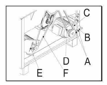
Take away the dismountable machine side covering. By means of 2 nuts (A) at the tightening screw (B) change the position of machine holder(C) deflecting so as the V-belt of cutterblock drive (D) is sufficiently tightened. Fix the position again by tightening the nuts. After loosening of screws (E) do shift (in slots) the feeding drive motor so as the V-belt (F) is sufficiently tightened. Tighten the screws again and put on the removable covering.
