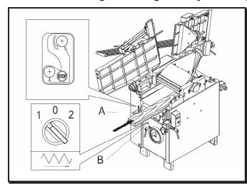
In case the machine is equipped with feeding drive by friction - gearing, start/ stop the feeding with lever (A). Feeding is on, if the lever is in upper position, feeding is off, if the lever is in lower position.
