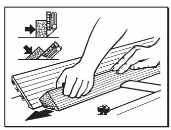
Check the angle of the longitudinal ruler at loose tightening levers (the position 90° is fixed), tighten levers again and switch on the machine. Push chamfered workpiece forwards and against the ruler.
