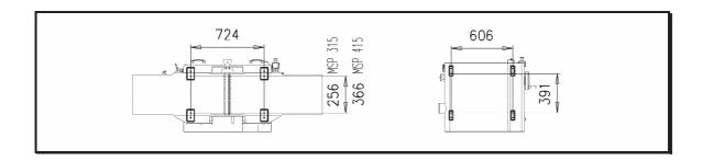
The machine (in lower part of stand) has feet with levelling screws and bores for anchoring bolts. Use steel washers (part of delivery) under levelling screws and balance the machine in plane with the clearance limit 1 mm/1metre
