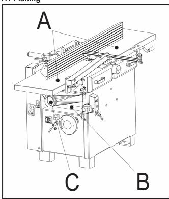
Both planing tables (A) have to be closed when planing. Suction hood (C) is flipped under to the back planing table and thicknessing table. To have enough space between these two tables is necessary to come down with thicknessing table on the value 160mm according to the scale. Suction tube must be connected to outlet (C)
