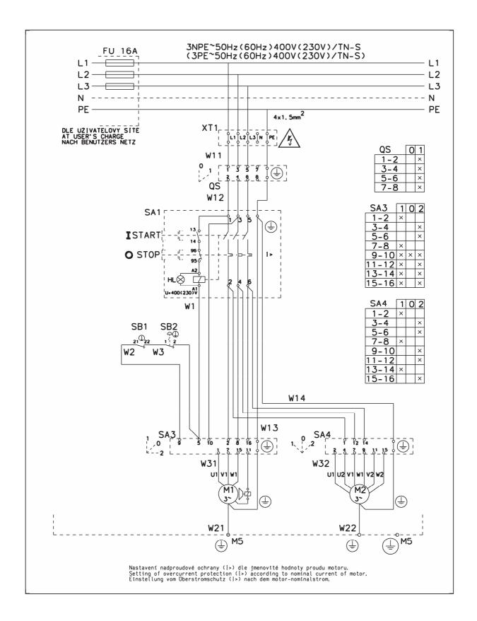
**Diagram 020-3-2** (3,0/3,7 kW, 3x400 (230) V, 50 (60) Hz, main switch, connection box, stop-button, reverse, brake release, two speed feeding motor)
