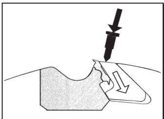
Discharge the knife in the cutter-block by knocking with accessories hammer onto the gasset.
