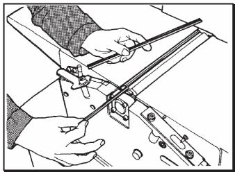
Take the blunt knife out from cutter-block and replace it with a new one.
