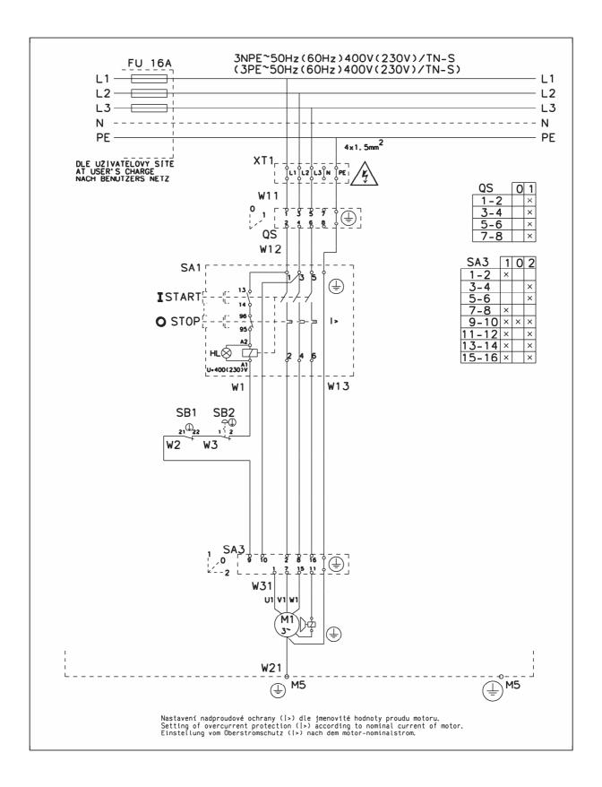
**Diagram 019-3-2** (3,0/3,7 kW, 3x400 (230) V, 50 (60) Hz, main switch, connection box, stop-button, brake release, two speed feeding motor)
