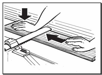
Put the flat piece on the planing table, take up the roller cover by left hand, adjust it to required height about 5 mm over input workpiece and switch on the machine. Push the workpiece towards the cutterblock, your hand is moving over the cutterblock cover, the workpiece is being shifted by hands - not by your entire body!
