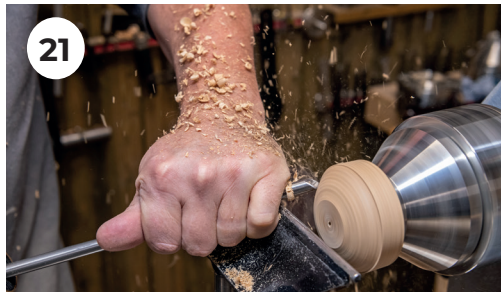
21. Once the important measurements have been turned you can have some fun with the shaping, I'm using an Ogee design on mine which has a nice convex turning into a concave at the bottom.
