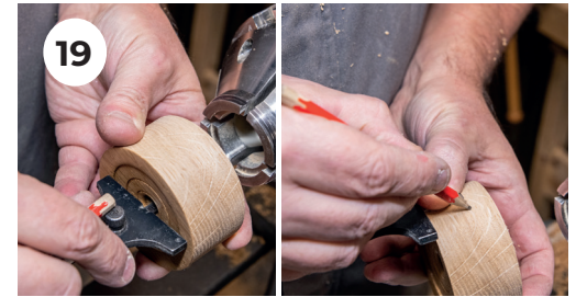
19. Double check your 10mm measurement with a depth gauge and mark this on the outside of the base. Hold the screw against the measurement to make sure all is correct and if not, it can be corrected on the front face.
