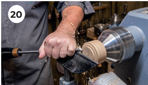
20. Holding the blank via its recessed base, turn down to the finished thickness.
