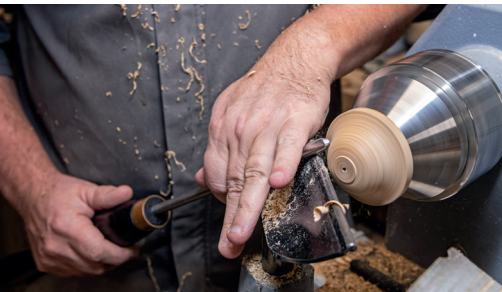
21. Once the important measurements have been turned you can have some fun with the shaping, I'm using an Ogee design on mine which has a nice convex turning into a concave at the bottom.
