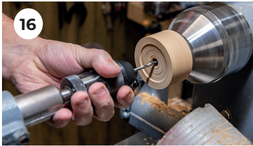
16. Now drill all the way through the blank with a 4mm drill bit to allow the thread of the screw to pass all the way through.
