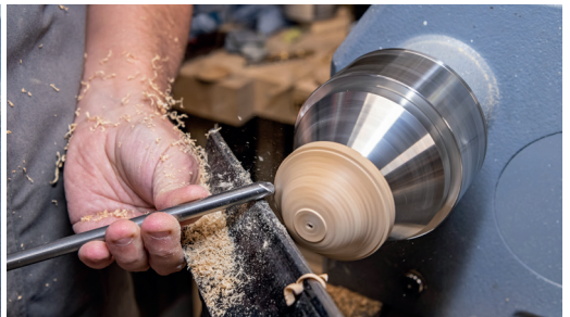
19. Double check your 10mm measurement with a depth gauge and mark this on the outside of the base. Hold the screw against the measurement to make sure all is correct and if not, it can be corrected on the front face.
