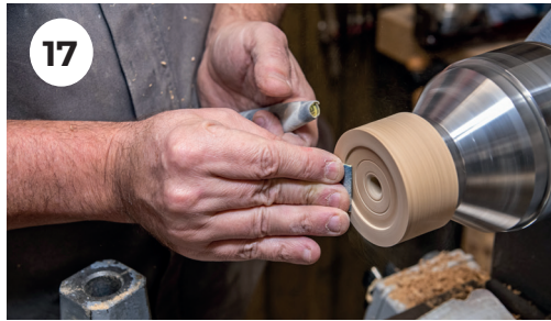
17. The base can now be sanded to a finish.
