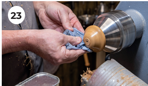
23. Oil the finished surface and buff with polishing cloth.
