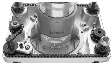
Router/mounting plate mounted in the router elevator
