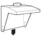
Place Varivac canopy around the outer rear top of the Ceramic Chip Forge and bolt through the corresponding holes in both units.
