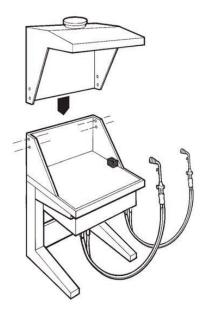
Place Varivac canopy around the outer rear top of the Ceramic Chip Forge and bolt through the corresponding holes in both units.
