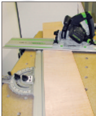
Fit the lever cramps in the tabletop holes to clamp a horizontal workpiece
