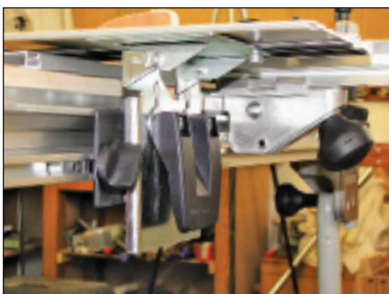
The height of the guide rail support brackets can be easily adjusted and locked
