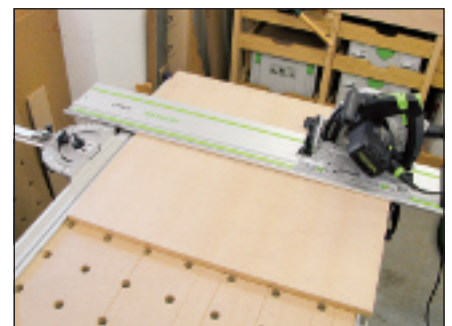
The guide rail and back stop allow you to cross-cut work up to 700mm wide
