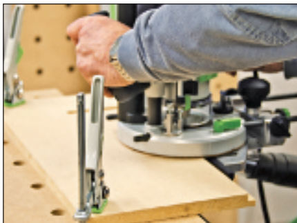
Fit the lever cramps in the tabletop holes to clamp a horizontal workpiece
