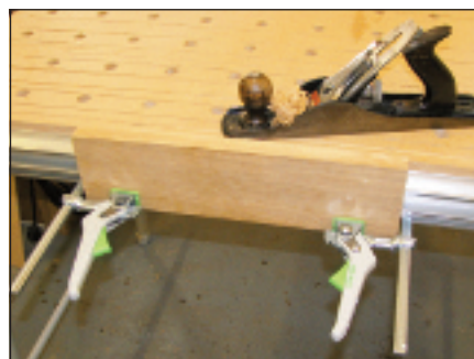
You can also fit the lever cramps in the T slots on the side to act as a vice
