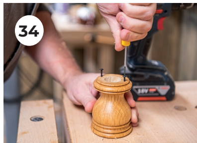
34. Before adding the mechanism screw the screws and remove them to cut the thread.
