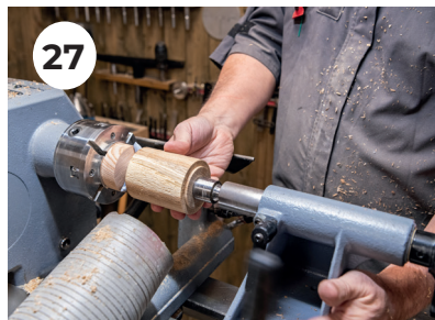
27. Bring the tailstock up and hold between centres, using the through hole to centre on.
