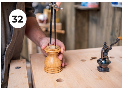
32. Transfer this measurement to the top of the grinder base and push in to create a shallow hole where you will need to drill.
