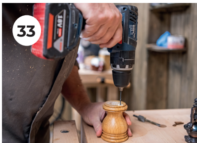
33. Using a 1mm drill bit, drill a shallow hole to except the fixing screws.
