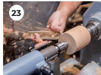
23. Remove the blank from the lathe and prepare a blank to drive the project by roughing a piece of scrap wood down to a cylinder.
