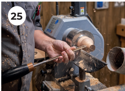
25. Turn the blank down to a concave cone shape.
