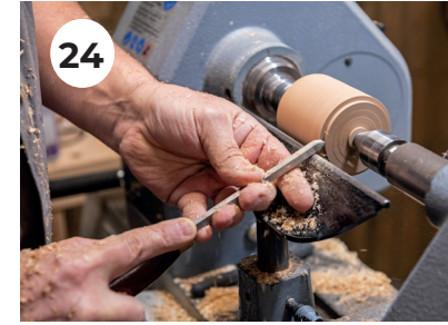
24. Create a hold point and hold in the chuck.
