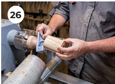
26. Add a piece of tissue to the cone and insert the project blank over the cone.
