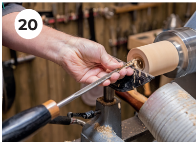
20. Using your bowl gouge, turn a radius toward the through hole.
