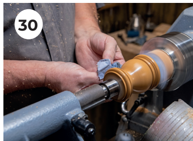
30. Give the whole project a finish of food safe oil and remove from the lathe.
