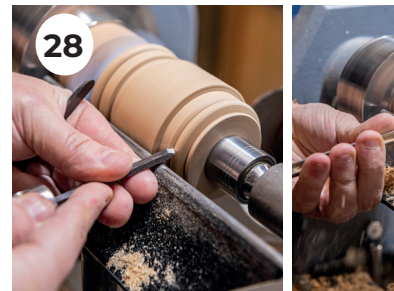
28. Now the blank is secure and both top and bottom have been finished, you can turn your chosen outside form.
