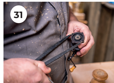
31. In preparation to screw the mechanism onto the base, use a set of dividers to measure the centre spacing of the fixing holes.
