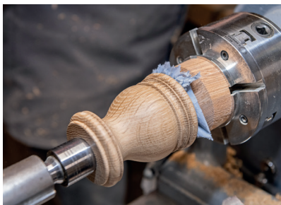
26. Add a piece of tissue to the cone and insert the project blank over the cone.
