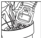
**Determining the moisture content of soil**
