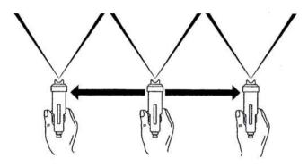
Start moving the spraygun in the direction you want to spray and press the trigger. Between each successive pass, overlap by about a quarter.
